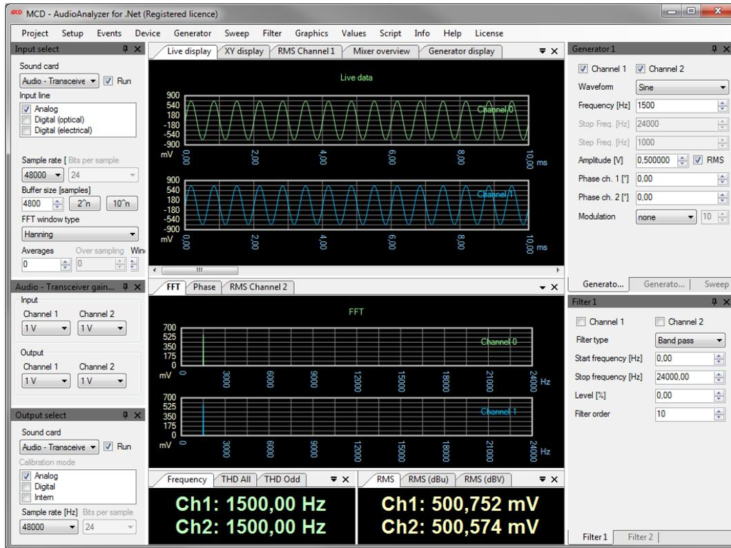
Figure 6: User Interface of the Toolmonitor AudioAnalyzer
