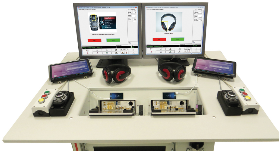
Picture 2: Manual Functional Test with two operating stations.
