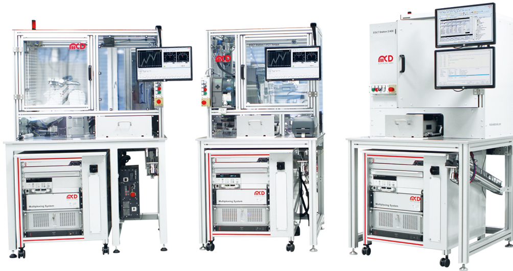
Picture 1: The test cell with a 6-axis robot for rotative test of rotary switches on the left, the station for examination of power window modules in the middle and the AOI station on the right.
