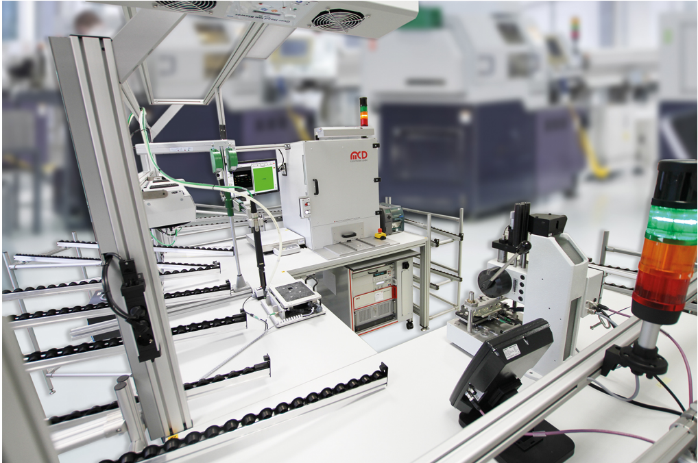
Picture 3: In the foreground (right) the hand-operated press for panel assembly, (center) the station for final assembly of the control unit and in the background the test cell for optical and electrical testing.
