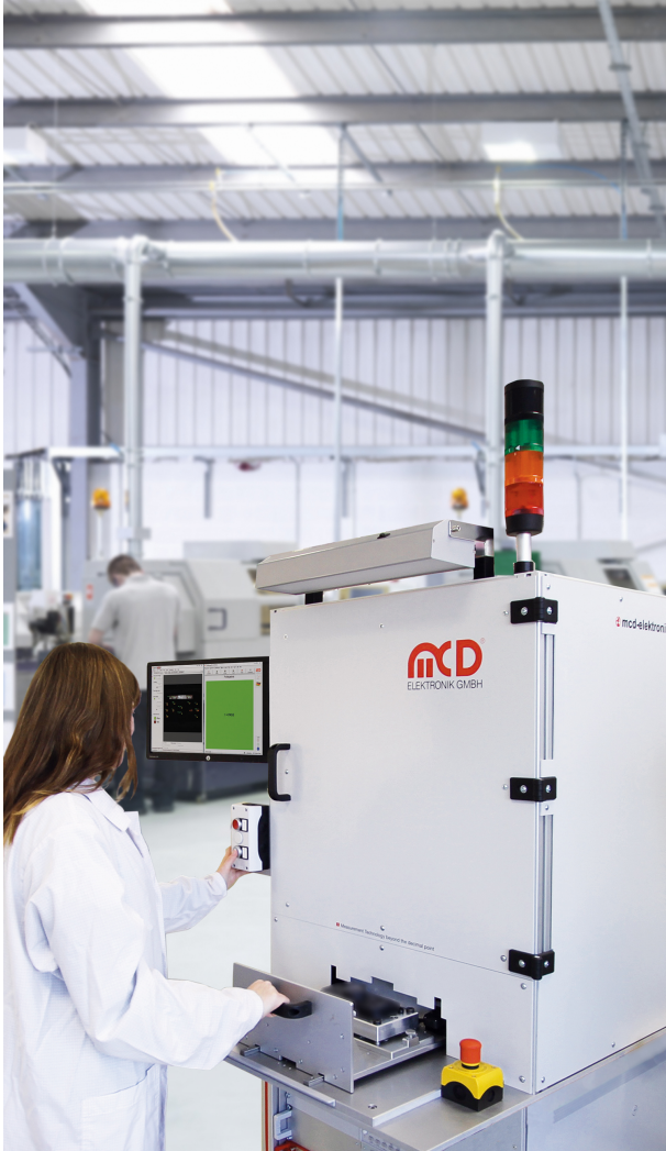
Picture 2: Placing a module in the test cell tray.
