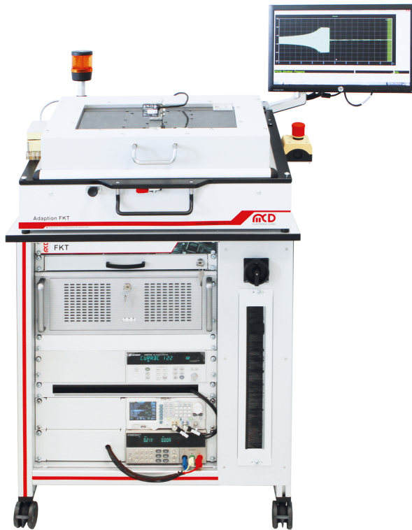
Picture 1: The test station with adapter for the DUT and monitor for the user guidance. On the monitor: the oscillogram of the ignition impulse for the lamp.
