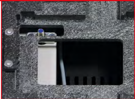
Blue Position Sensors inside of the Desktop Station
