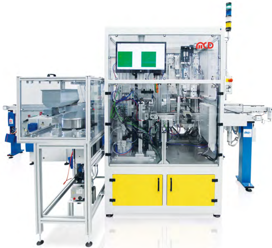
Supply and Assembly of a Seal Ring and Leakage Test
