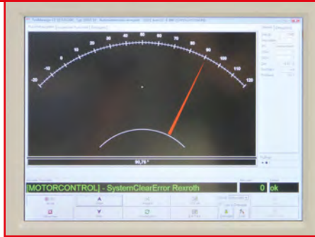
Monitoring of a Triggered Rotation Angle while Testing
