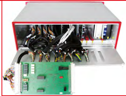
UMS1300 with Connected ULC Measurement Card
