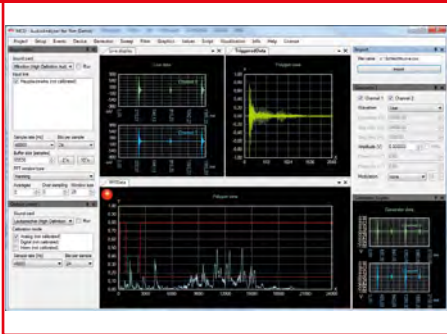
Analyzing the Clicking Sound of a Defective Flasher Relay
