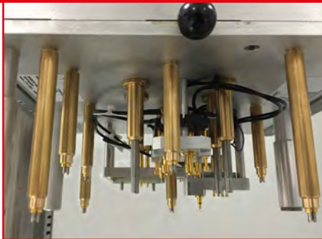
Downholder with RF Contacting
