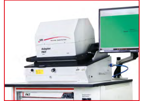
Shielded RF hood for Functional Testing of Signals
