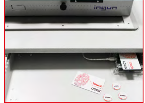
RFID Cards as Chip or Card Variations with Receiver Module
