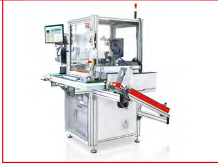
EOL Test System with integrated LED Visualization of Test Results
