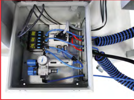
Pressure Station with Filter Regulator, Valve Terminals and Pressure Sensors
