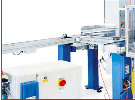
Automatic Feeding of DUTs to Test Station via Transfer Belt
