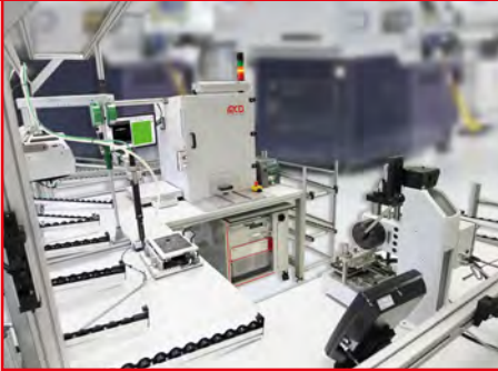
Assembly Station with Manual Hand Press and Screwing Station
