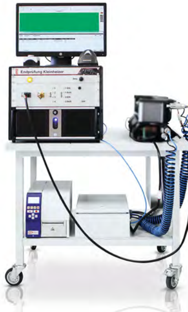
Quick Connector for Pneumatic DUT Contacting
