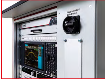
Spectrum Analyzer during Process of Testing WiFi and ZigBee Signals
