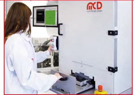
Functional, Optic and Haptic Test of Operating Elements
