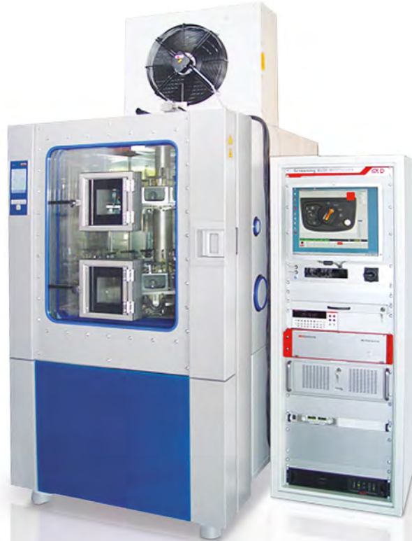
Rotating Carousel inside Climatic Chamber
