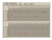
The check box 'ENLed on' activates the Enable LED of the card i.e. important for debug purposes. The button 'Reset' sets back the error logic of the card.
