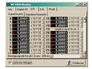
impedance of the source signal is too high, then the measuring channel has very less time to swing at the right value. It can thus lead to a wrong measurement. However the load on the system is reduced when shorter settling time is used. Only those channels marked with green tick symbol cane read back in a cyclic manner. By clicking on this green symbol the activity of the channel can be changed.
