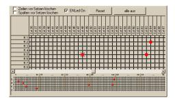
occur by a wrong connection due to any previously made row or column connection. The delay time set by the progress bar 'Break-before-make delay' waits for the set time before activating the relays. The button 'Clear all' deactivates all connections.
