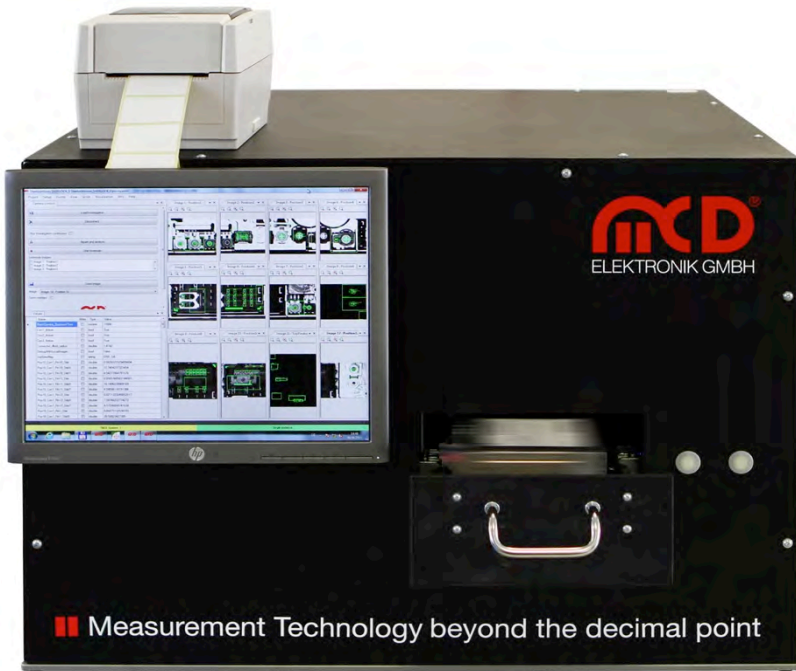
Image 2: MCD Sherlock Vision applied to the testing of infotainment systems.
