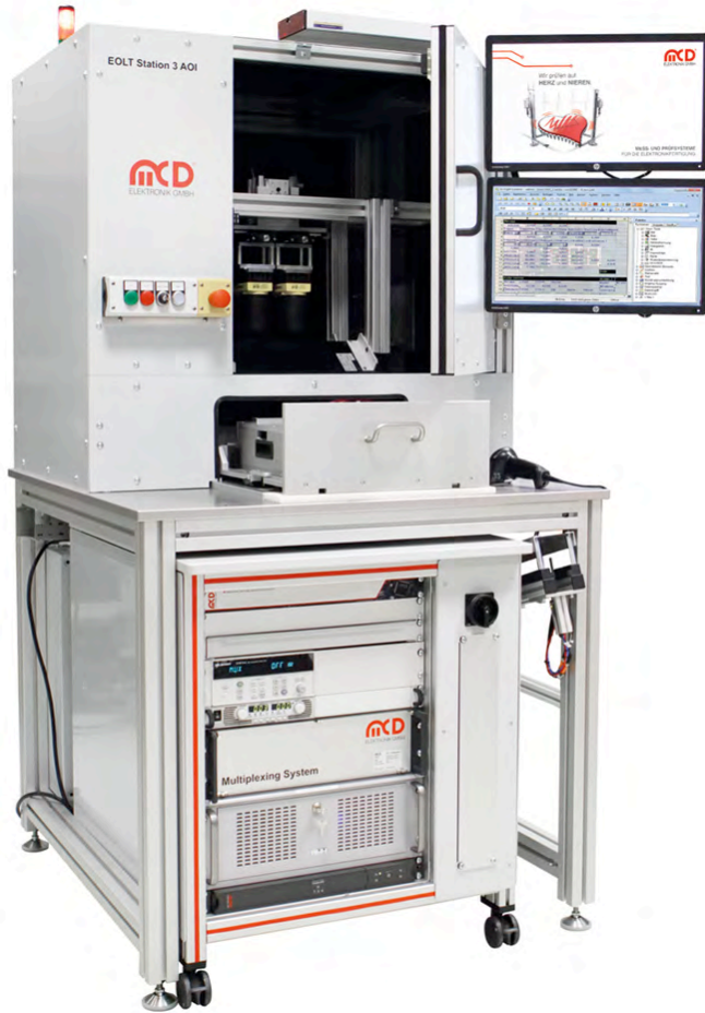
Image 1: The optical test station MCD COGNEX Vision with an inside view to the open camera area.
