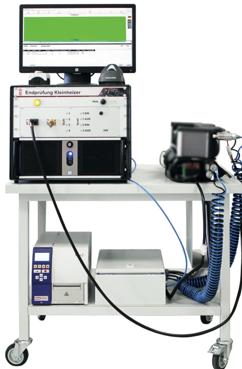
Picture 1: End-of-Line test system for floor heating systems.
