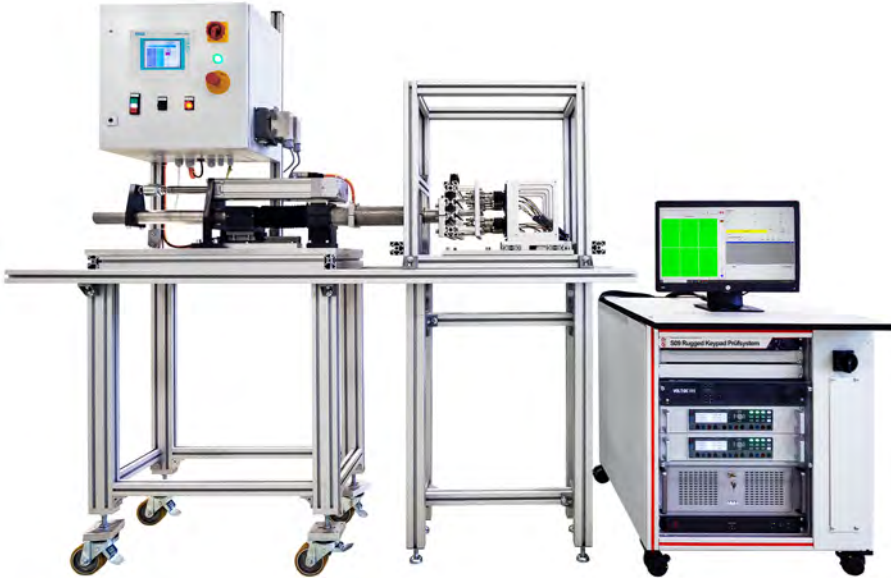
Picture 1: Durability test station for the testing of rugged keypads from heavy duty and special purpose machines.
