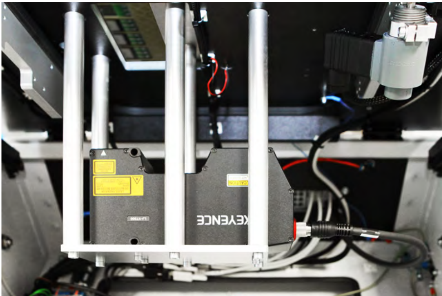
Image 2: Positioning of IGBTs is qualified by a Keyence laser profiler with an accuracy of 0,005 mm.
