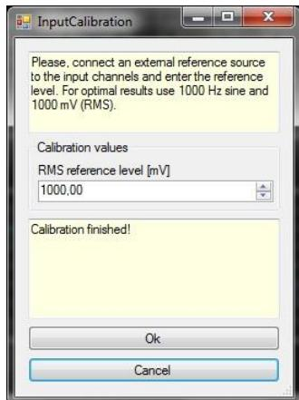
Figure 36: Input Calibration
