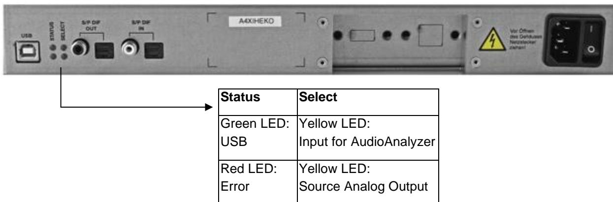
LED input for AudioAnalyzer (yellow): Shows the selected source for the AudioAnalyzer (USB).
