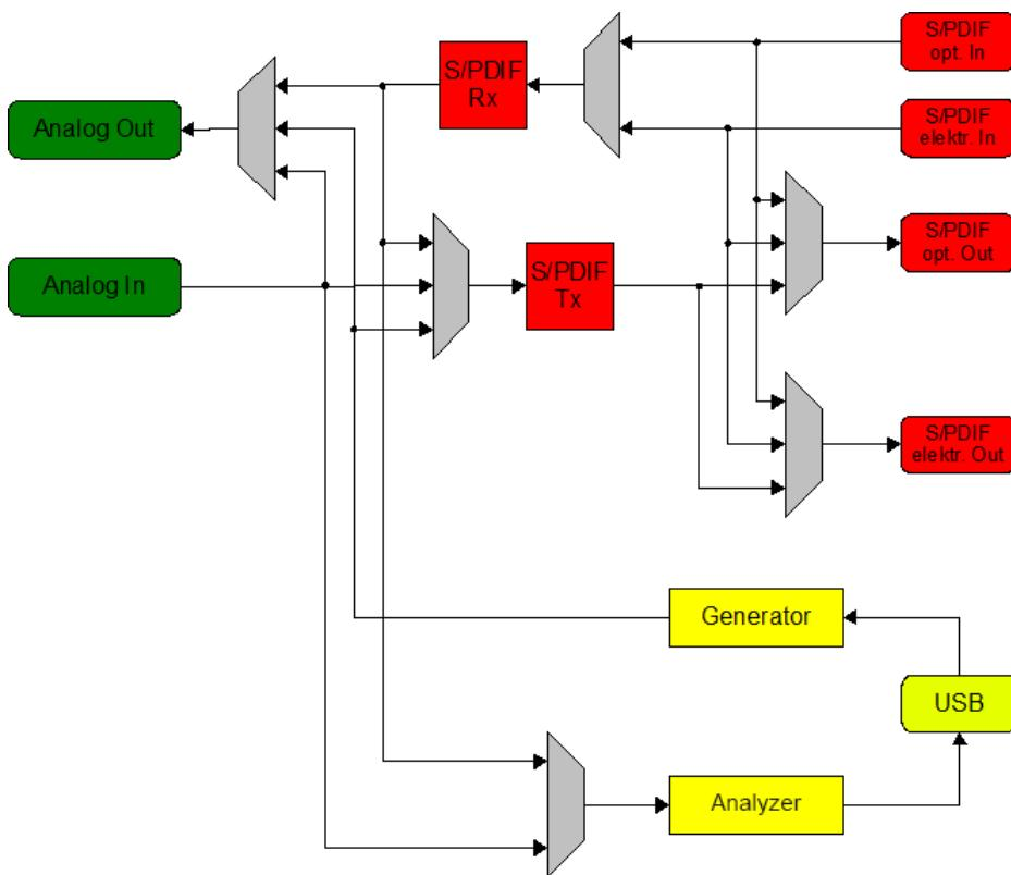
Figure 39: Block Diagram
